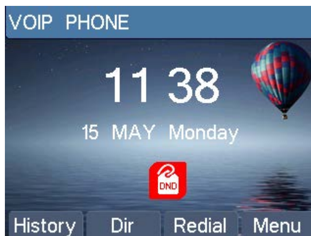
Figure 56 - DND Enabled on All Lines
